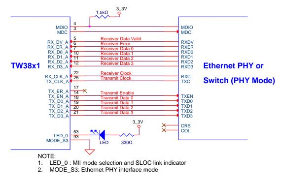
FIGURE 12. MII INTERFACE WITH ETHERNET PHY
