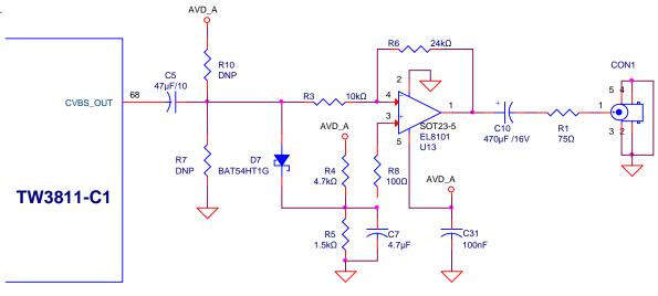
FIGURE 10. LOW-COST CVBS OUTPUT CIRCUIT
