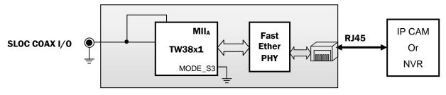
FIGURE 3. ETHERNET PHY INTERFACE MODE FOR DONGLE SOLUTION
