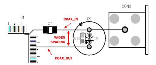
– Don't make a "T" as shown below. This degrades return loss and may reduce maximum COAX cable length.
