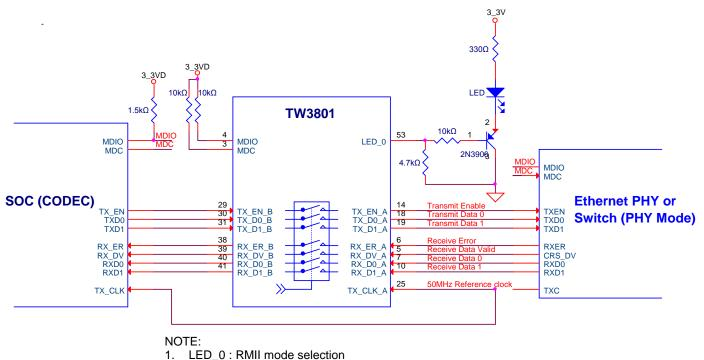
The RMII connections for pass-through mode are shown in Figure 7.
