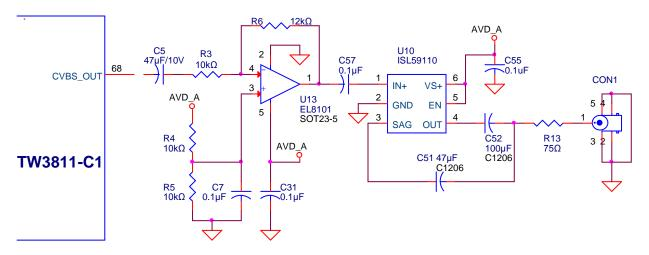
FIGURE 11. BETTER CVBS OUTPUT CIRCUIT
