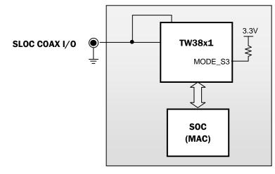
FIGURE 4. SOC INTERFACE MODE FOR EMBEDDED SYSTEM
