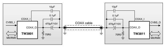
FIGURE 2. SLOC COAX I/O CONFIGURATION
